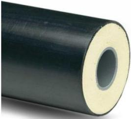
COOL-FIT ABS Plus pipes are made of ABS raw material. The insulation made of PUR foam provides excellent insulation properties, protected by a UV and weather-resistant PE outer jacket.
