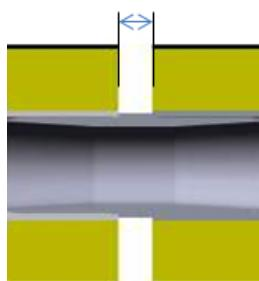
Each of these COOL-FIT ABS Plus connections creates a gap of 10 mm. The gap is used for visual inspection during the pressure test and is closed after a successful pressure test.
