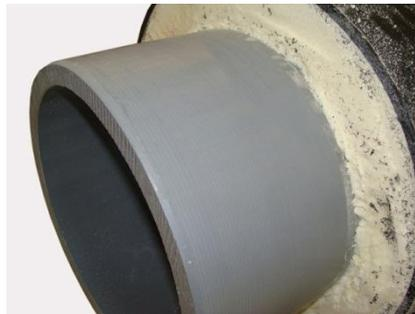
After peeling, the surface is free of PUR.
