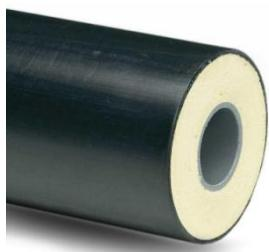
COOL-FIT ABS Plus pipes are made of ABS raw material. The insulation made of PUR foam provides excellent insulation properties, protected by a UV and weather-resistant PE outer jacket.
