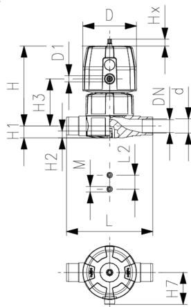
**Diaphragm valve DIASTAR Six ABS****FC (Fail safe to close)****With solvent cement spigots metric****Model:**
