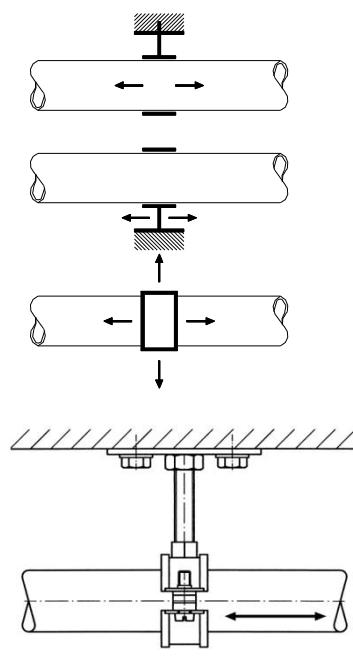
When installed, the inner diameter of the bracket must be larger than the pipe outer diameter to allow for a change in pipe length at specified locations. The inner edges of the brackets must be constructed in such a way that the pipe surface cannot be damaged.
