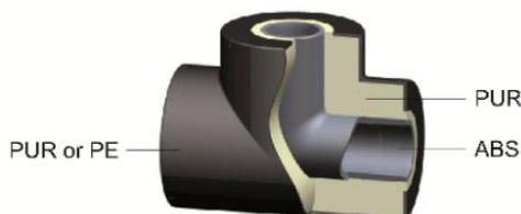
The ABS fittings used in COOL-FIT ABS Plus are made of the same raw material as the pipes. The insulation made of PUR foam is protected by a PUR or PE outer jacket. This makes the fittings fully compatible with COOL-FIT ABS Plus pipes.
