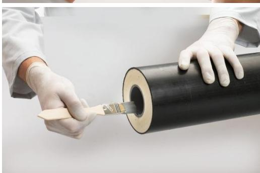
Apply ABS cement of approx. 1 mm thick onto the cementing surface of the nipple.
