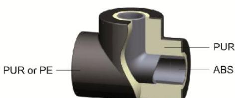
The ABS fittings used in COOL-FIT ABS Plus are made of the same raw material as the pipes. The insulation made of PUR foam is protected by a PUR or PE outer jacket. This makes the fittings fully compatible with COOL-FIT ABS Plus pipes.
