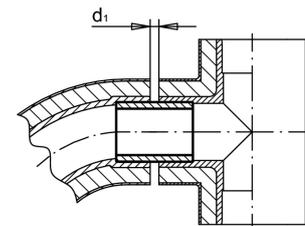
**COOL-FIT ABS Plus Barrel nipple d-d PN10**
