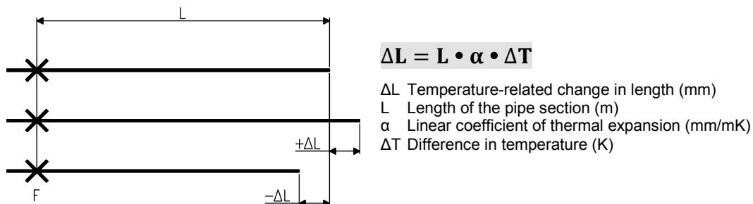
The following temperatures must be known to calculate the change in length  $\Delta L$  (mm) of the COOL-FIT PE Plus pipe:
