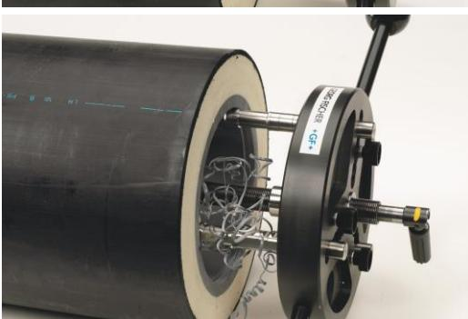
Screw in the cutting head, check the cutting knife and the two guide heads for correct seating.
