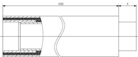
The peeling length depends on the ABS pipe diameter. The following formula is used for the calculation:
