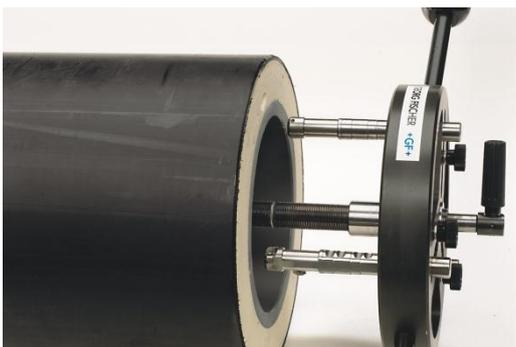
Fix the tool in the pipe with the clamping elements.
