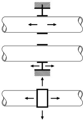
When installed, the inner diameter of the bracket must be larger than the pipe outer diameter to allow for a change in pipe length at specified locations. The inner edges of the brackets must be constructed in such a way that the pipe surface cannot be damaged.
