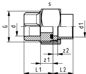
**Adaptor union ABS/copper for soldering metric**
