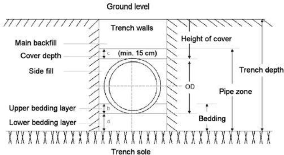
The pipe zone has to be designed according to planning fundamentals and static calculations. The area between trench sole and side fill is referred to as bedding. A load-carrying bedding must be created by using soil replacement. For regular soil conditions, EN 1610 specifies a minimum thickness of  $a = 150$  mm for the lower bedding. In addition to the minimum thickness, corresponding requirements are also imposed on the building materials that must be used for the bedding.
