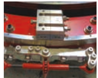
Swing bolts & hinge mechanism speeds assembly & mounting
