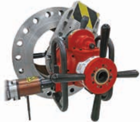
E.H. Wachs EP 424 End Prep with AutoFeed performs pipe end preps & flange facing
