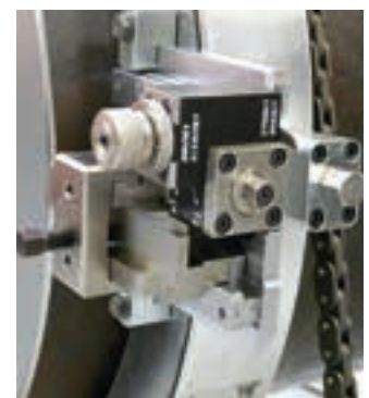
DynaPrep MDSF slides feature Rapid Adjust tool depth control
