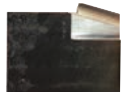
Counterbore tool taper 4:1
