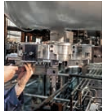
Compact, the FFC can face flanges in any position or orientation
