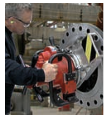
Faces flanges up to 36in (914 mm) with optional slide
