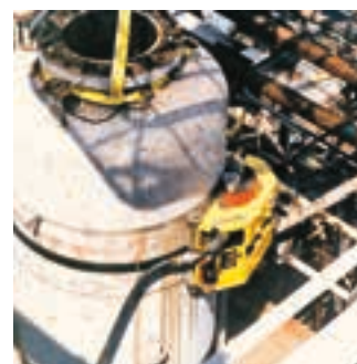
Add mounting chain sections to fit larger diameters
