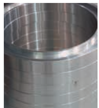
Machined split frame rings
