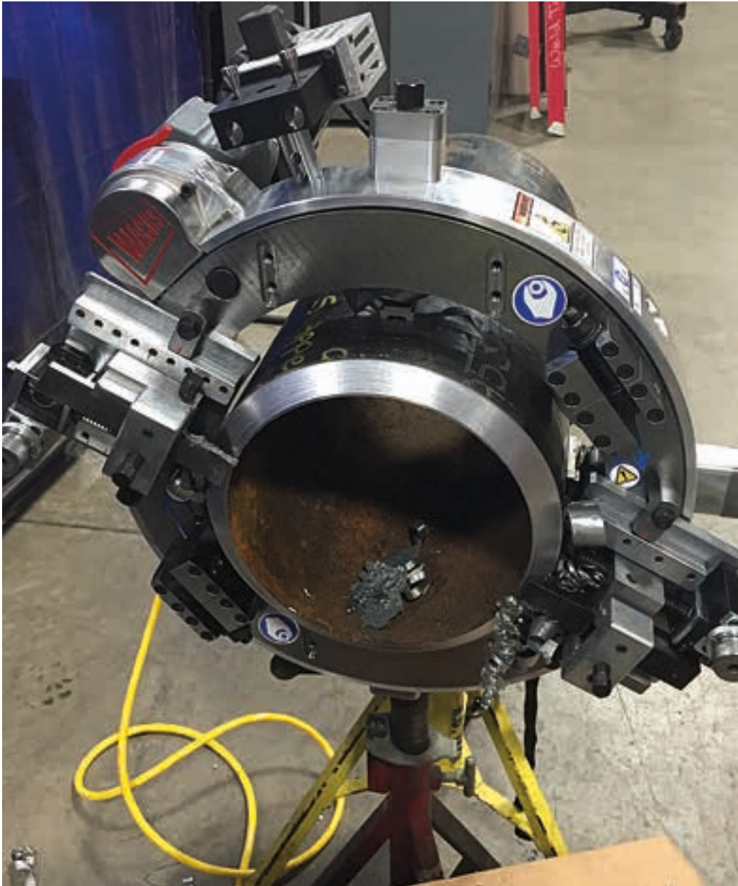
V-Lock ring mating surface resists force distortion
