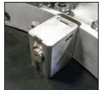
Leg extensions mount without removing machine from pipe
