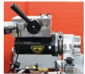
Tool-free quick mounting for fast setup and operation
