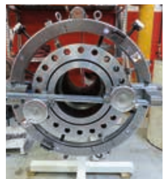
Two FFR modules performing simultaneous operations
