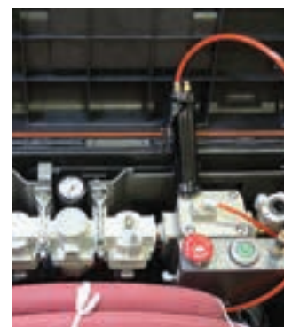
Ergonomic fingertip control with safety stop button
