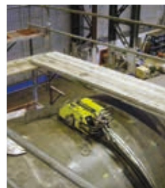
Trav-L-Cutter being used for submarine decommissioning
