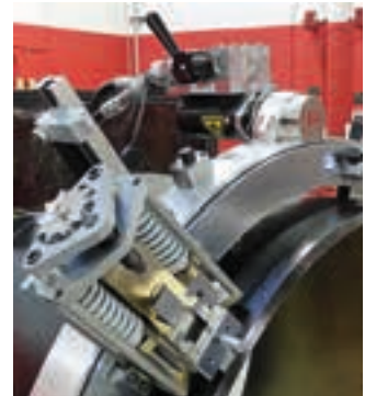
Out of round tracking slides are ideal for pipelines
