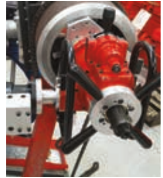
EP 424 single point deluxe beveling with form tool rotating head
