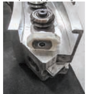
V-Lock ring mating surface resists force distortion
