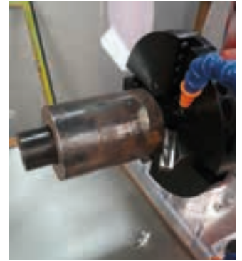
Weld Coupon loaded, ready for prep
