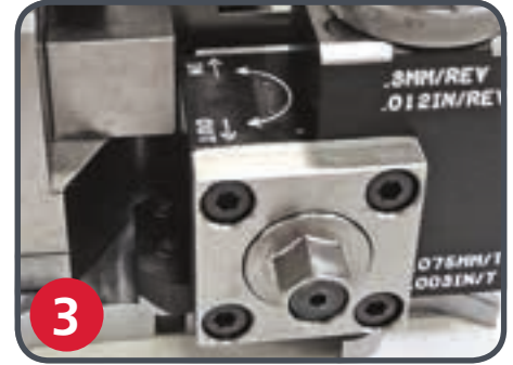
Rapid Adjust feature speeds positioning of tooling
