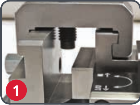
Accepts most popular tooling sizes including 1in (25.4 mm) square & 1/2x 3/4in (12.7 x 19 mm)
