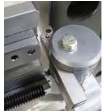
FFR tooling can be adjusted on multiple axes
