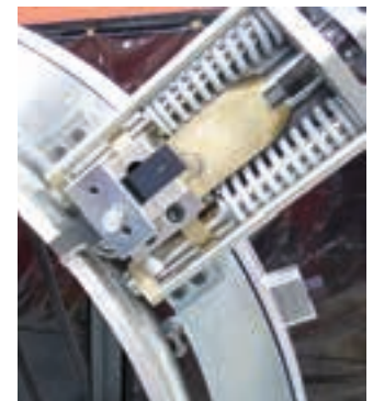
OD tracking slides follow out-of-round pipe & vessels.
