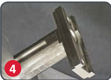
Ring sizes 20in & below use four clamping feet for squaring
