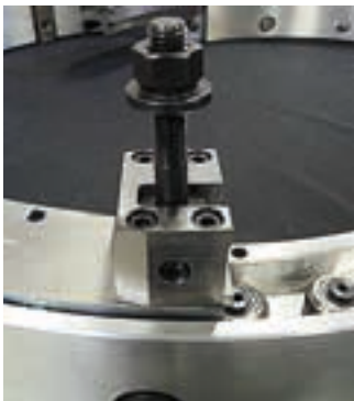
Aluminum stationary frame with steel rotating ring
