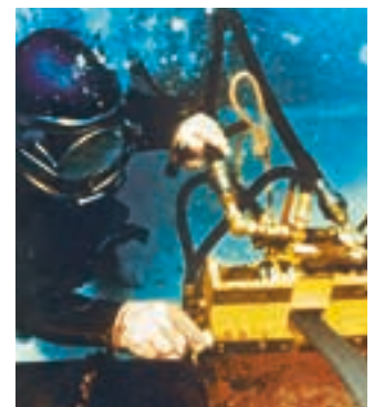
Model HE Hydraulic Trav-L-Cutter suitable for full immersion
